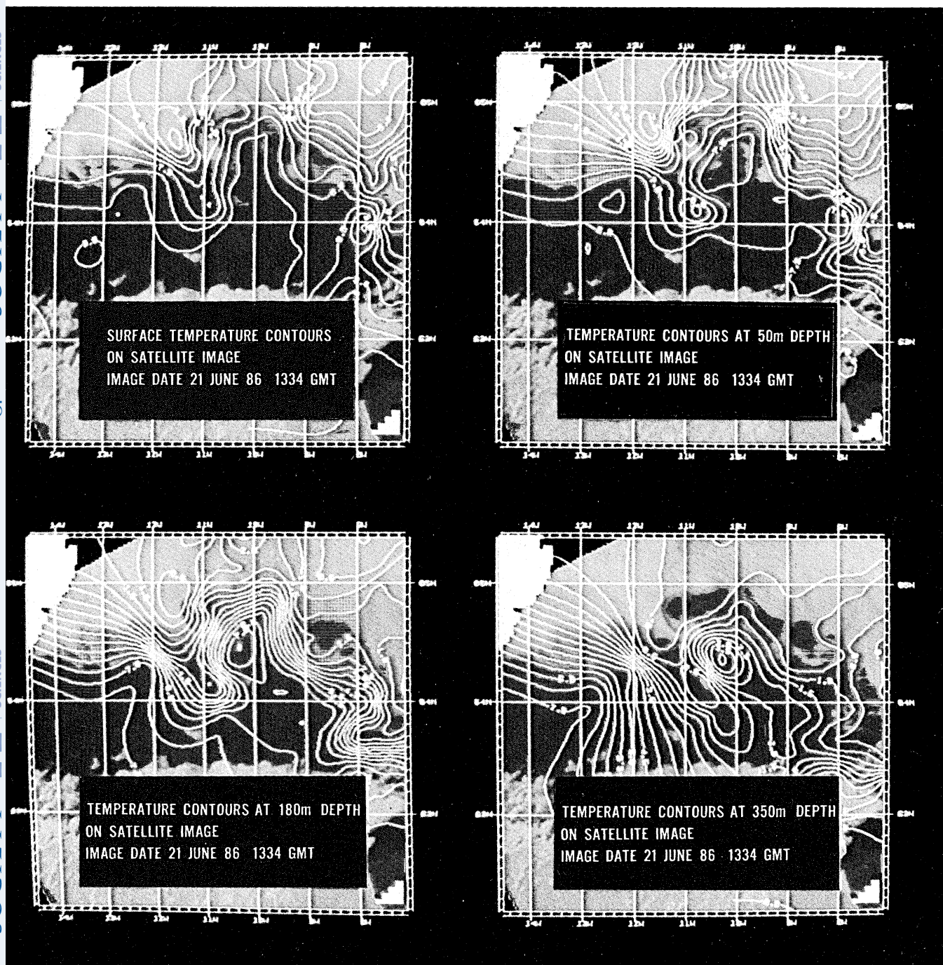
FIGURE 9. Contoured in-situ temperature data at significant depths of near-surface, 50m, 180m and 350m depth overlaid on the satellite subimage; an example of how in-situ data can be compared with accurately registered and atmospherically corrected satellite images.
